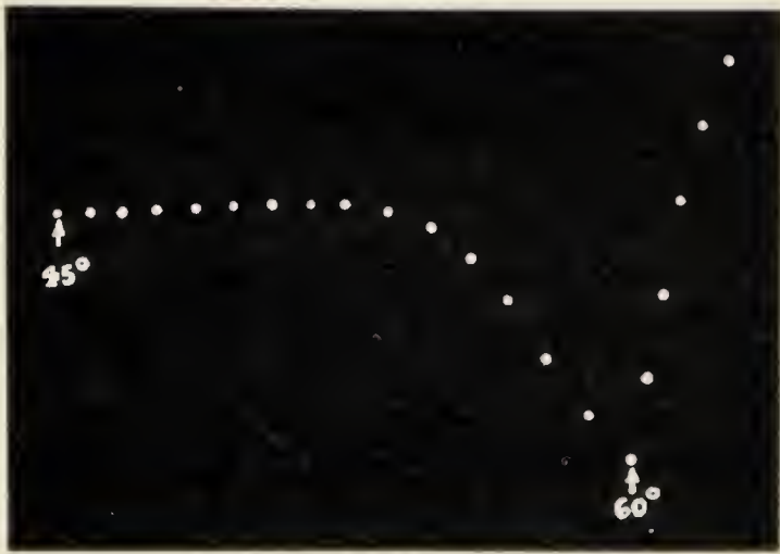
FIG. 131. Record of variation in weight of Carissa fruit under rise of temperature ( 45^{\circ} – 60^{\circ} C.). Note abrupt inversion of the curve at 60^{\circ} C., indicating a sudden increase in weight.
